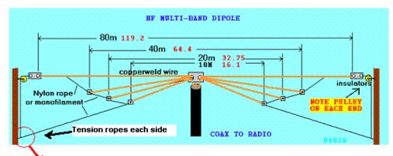
Tension rope is not tied to pully rope in picture. It is tied near location of pully rope down on supports within easy reach. It is tied last after final SWR adjustment and the antenna is in it's final position.
