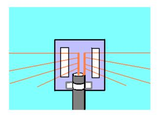
The white areas in the center support drawing above are mechanical supports, clamps, wire ties or whatever your genius can come up with to support the main (top wire) and the weight of the coax.
